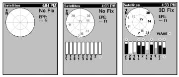
Satellite Page. First page (left) indicates unit has not locked on to any satellites and does not have a fix on its position. The second page (center) shows satellites being scanned. The last page (right) shows satellite lock-on with a 3D position.
